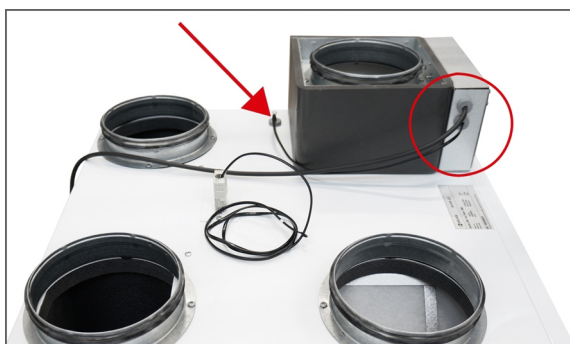
5. The temperature sensor for the preheating surface is pushed 8 cm into the tulle. Then, inside the unit, it can be seen hanging just above the outdoor air filter.
